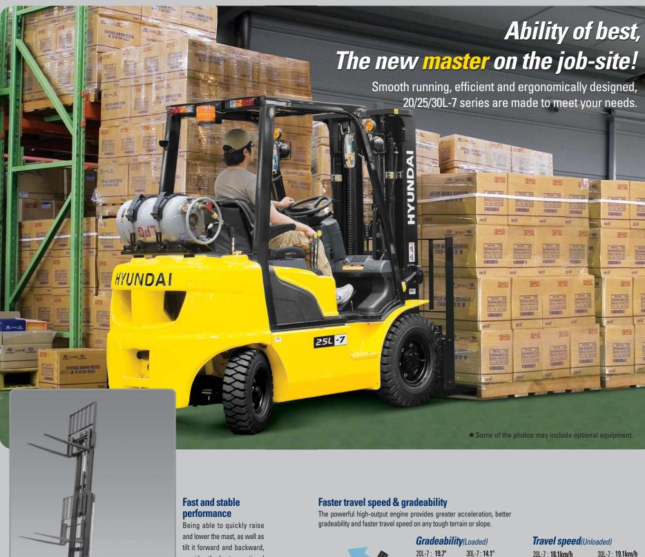
Being able to quickly raise and lower the mast, as well as tilt it forward and backward, provides the best operational conditions during unloading. When the truck is fully loaded, mast lowering speed is carefully controlled to ensure safety by the down control valve.
