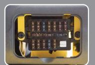
An accessible, compact fuse box for easy inspection
