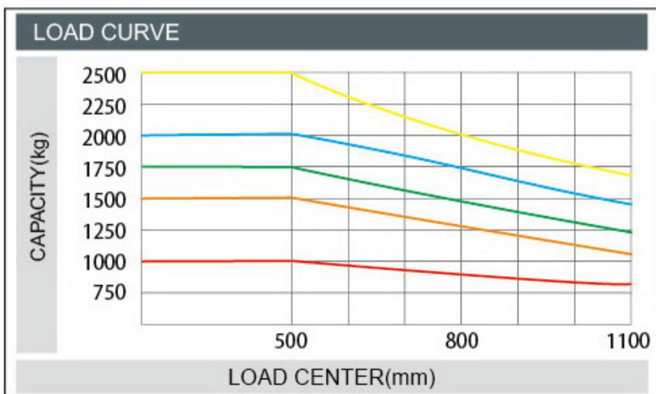
**Note:** The vertical axis stands for load capacity and the horizontal axis stands for load center which is calculated from the front surface of the forks to the gravity of the standard load. The standard load means a cubic with 1000mm edge length. When mast is tilted forward, using non-standard forks or loading large goods, the load capacity will be reduced. The load capacity of standard mast at different load center can be known from this load chart.
