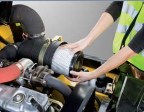
Easy change air cleaner The air filter is readily accessible for cleaning or replacement. (7inch Cyclone Type)
