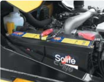
Double battery installation
