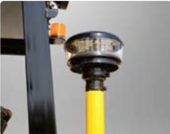
Visible precleaner Efficient, accessible pre-cleaner provides for longer engine life
