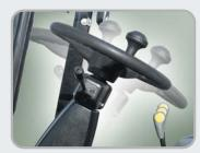
**Adjustable Steering Wheel** Steering wheel can be adjusted by a lever on the right-hand side for the most comfortable operator position.
