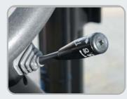
**Multi-Functional Switch** Integrated multi-functional switch lever enables the driver to operate lights and horn conveniently.
