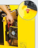
**Battery Disconnect Lever** / Switch
